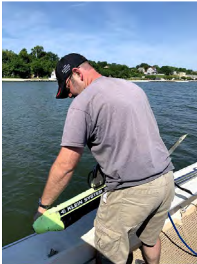
JRS May 2019 survey, diver lowers sonar towfish into the water.
